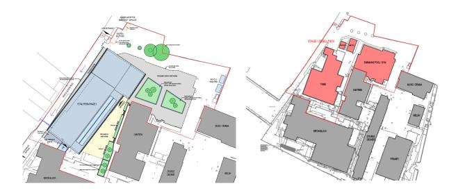
The footprint of the building shown on the plan on the left, with the existing buildings to be demolished on the right, highlights how the reduction on floor space, accommodates additional areas of open space and play area.
