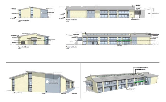
The use of brickwork as the predominant external material provides a clean and hardwearing finish, but complemented with areas of cladding, provides an inviting and well balanced appearance. The brickwork will complement that used within the existing school buildings.
